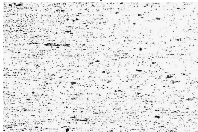
a – 1.20 % Ti and 0.028 % N; б – 1.20 % Ti and 0.287 % N; c – 0.35 % Ti and 0.182 % N Figure 1 is microstructure of the experimental thin-walled rolling from steel 13X12M2TБΦP with different content of titan and nitrogen (x 125)
