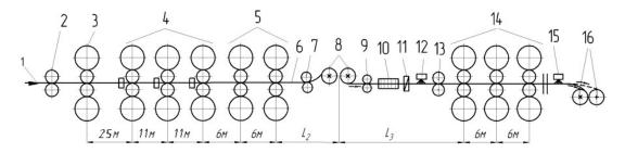
1 is slab; 2 is a descaler; 3 is a draft cage «quarto» (universal cage); 4 are universal draft cages «quarto» with vertical rollers; 5 are draft cages «quarto»; 6 - intermediate breakdown-bar; 7 are sending rollers; 8 - IRE with a hratsaving screen (drum reels); 9 are draw rollers; 10 is a pusher induction furnace; 11 are cuttors; 12 is a spraying device; 13 is a clean descaler; 14 is a continuous clean group of cages; 15 is a spraying device of ready band; 16 - coiler of ready band
